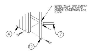
Figure 4. Attaching the side walls
